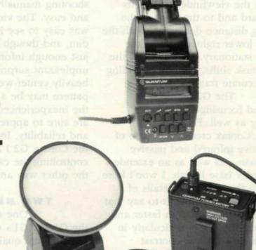
The base of the Qflash has an LCD display panel that provides a variety of information about setting up your flash and monitoring its functions. The first row of buttons includes the flash-fire, light, mode, and set functions. The mode button sets the flash up for manual, auto, TTL, or stroboscopic operation. Once you have selected a mode, you can then fine-tune your selection with the up/down or set buttons.
